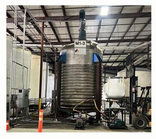
M1-3 Tank has Heating / Cooling coils for endothermic and exothermic reactions - 6,500 Gallon Tank Capacity
